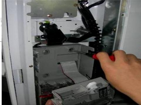
1. Press open the coin changer to move the reading head forward on the left card pin
