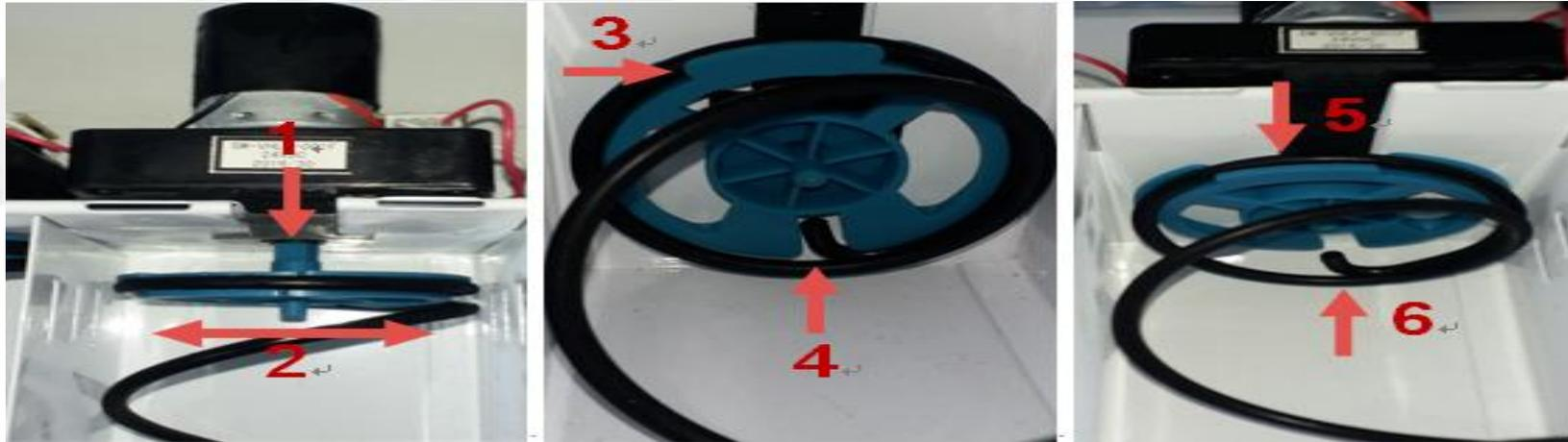
1. Hold and pull to detach the shank from the end of springs near the motor.
