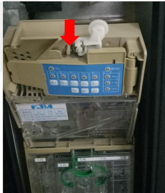
4. Pull out and remove the reading head.
