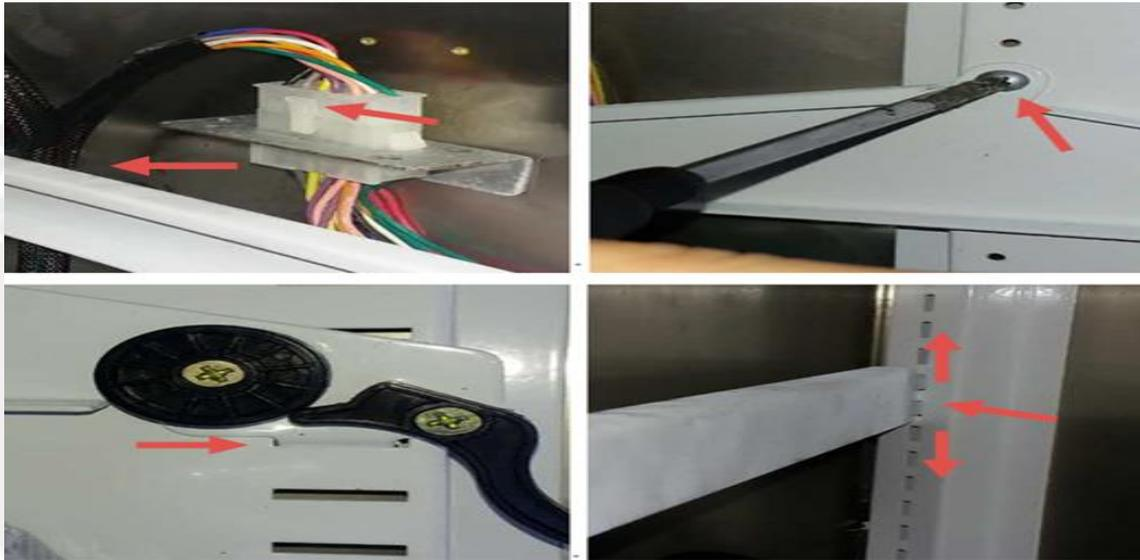
1. Pinch and pull out the buckle from its socket to disconnect the tray, and place it aside.
