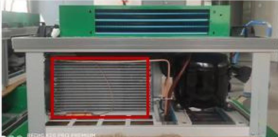
(The figure above shows the refrigerator, with condensation outlet circled out, which should be cleaned every two or three months.)
