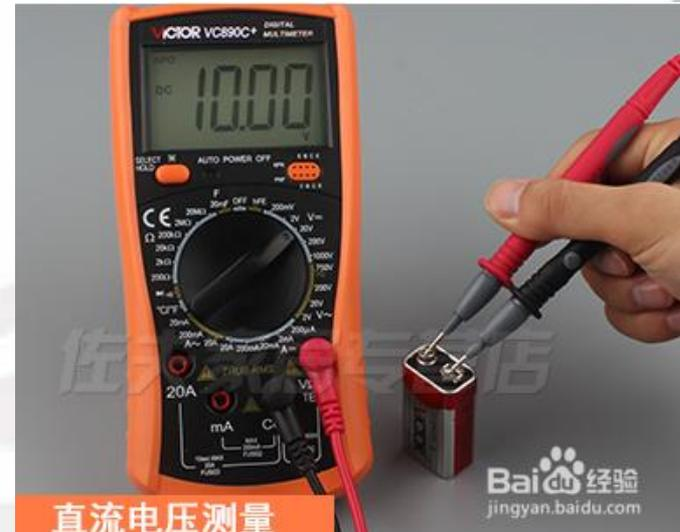
To measure the DC voltage, first set the gear to DC 200V, insert the red test lead into the V $\Omega$  and temp jacks, and the black test lead into the com jack, and start measuring the 9V battery voltage. The red test lead is connected to the positive electrode, and the black test lead is connected to the negative electrode. The measurement result is about 10V, indicating that the battery is in good condition.
