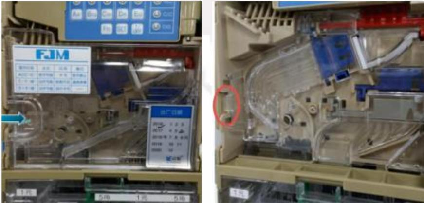
1. Push the handle in the direction that the blue arrow shows to open the lid.
