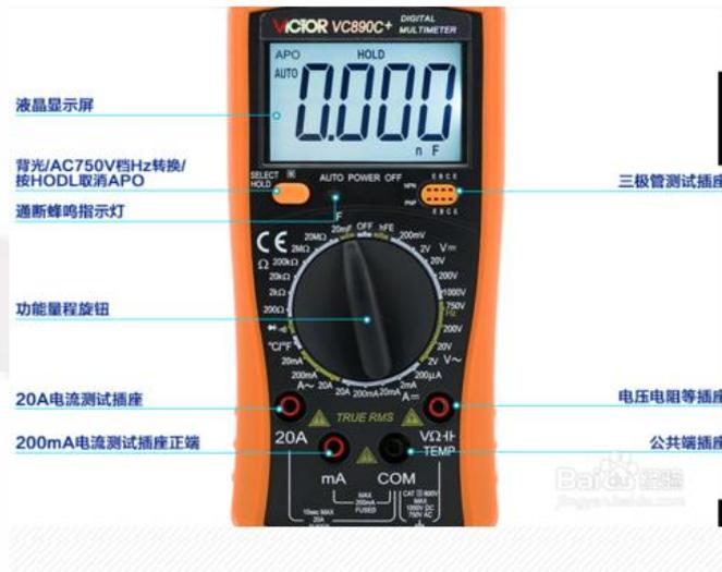
High-precision digital multimeter VC890D, the commonly used function buttons are as follows.
