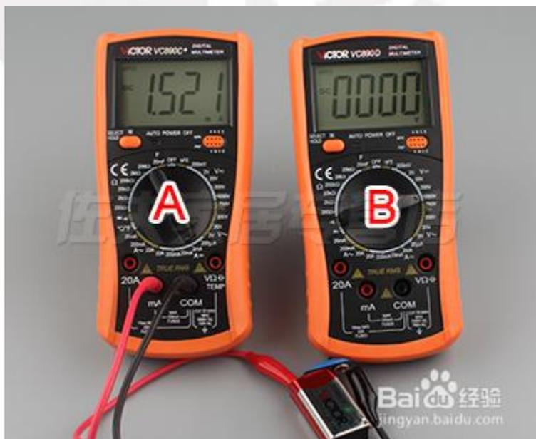
To measure the DC current, first set the gear to 20A and insert the red test lead into the 2mA jack. Then insert the black plug into the com jack, connect the multimeter in series with the circuit under test, and measure the current.
