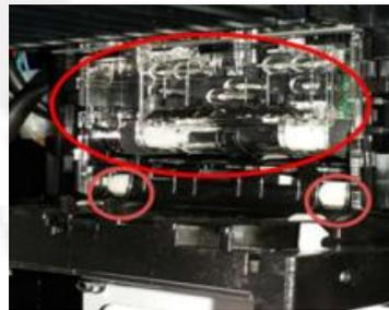
1. Push the lower bar and pull open the reading head of bill box.
