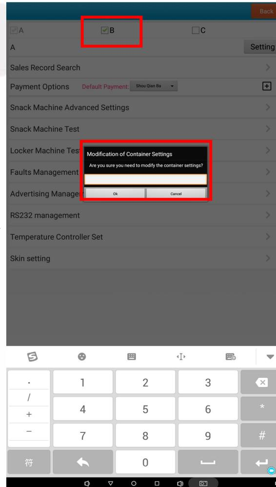
Tick the box marked B, key in the default password 352356, tap ok to finish the setting.
